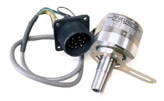
Our ST-EN-DR-ROD is a drop-in replacement for the Heidenhain ROD320 encoder. It is designed to provide precision feedback control for Siemens 1FT series Simodrive motors. It features a tapered shaft and custom flex mount. It comes in many line counts; 2,000,2,500, or 5,000 CPR,9" of cable and a 17 pin connector with the correct Heidenhain pinout.
